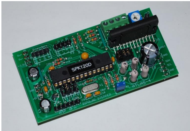
ATLAS-4 with TB6600HG driver for bipolar stepper motors operating up to 24 volts and 2.7 A.
