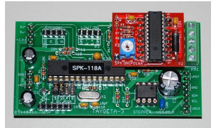
TAYGETA-3 with TB67S142NG driver for unipolar stepper motors, up to 14 volts and 800 mA.
